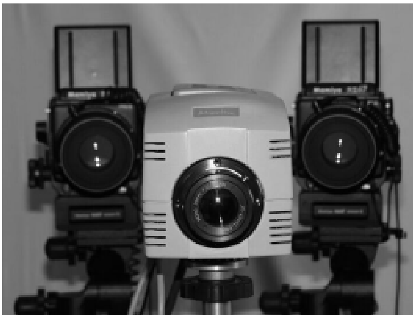
Figure 1: Configuration of the 3D thermogram scanner
