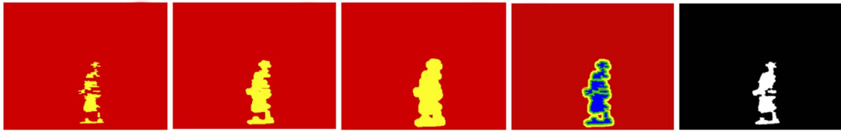
Fig. 6. Illustration of the definition of the three pixels sets used by the GrowCut algorithm. The first column displays the initial foreground set (f), the second and third column show the masks m1 and m2, respectively. The fourth column presents the three associated sets: foreground set (f), unlabelled set (u) and background set (b) are coloured in blue, in green and yellow, respectively. The last column shows the final foreground after growth. (For interpretation of the references to color in this figure legend, the reader is referred to the web version of this article.)
