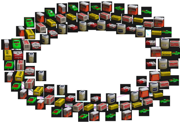
Fig. 7. The 1-dimensional joint view manifold embedded in the 2-dimensional space obtained by SLE with visualisation of corresponding objects.
