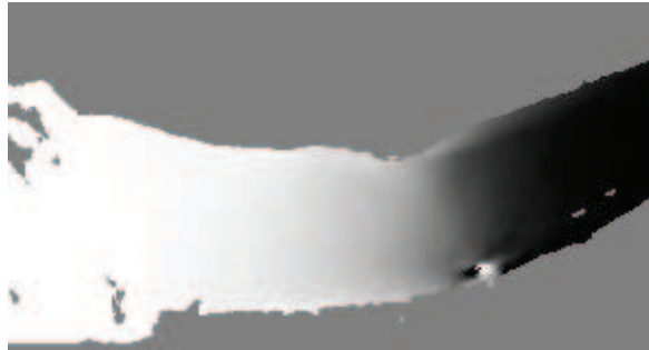
Figure 8. Weight distributed (a white value means w = 1 and a black one means w = 0 ).
