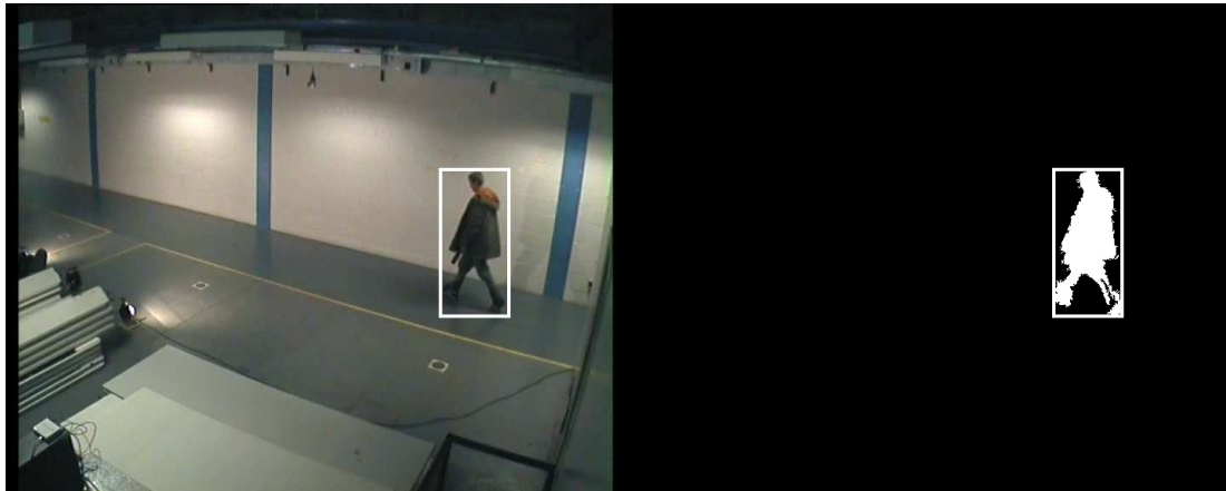
Figure 1: (a) The original image with the eventual ROI shown as a white rectangle, (b) the foreground after motion segmentation and shadow removal with the ROI shown as a white rectangle.
