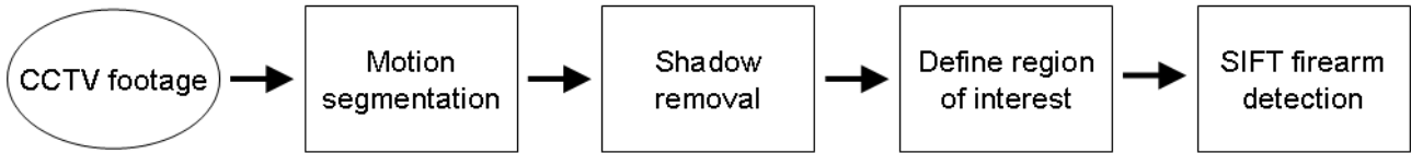
Figure 2. Summary of the firearm detection algorithm.
